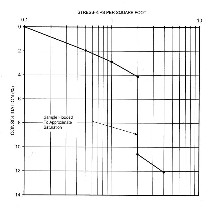
TEST HOLE NUMBER: 1 SAMPLE DEPTH: 5 FEET SOIL CLASSIFICATION: SM SOIL DESCRIPTION: SAND, silty MOISTURE CONTENT (%): 3.4 DRY DENSITY: 103 lbs/cu ft
